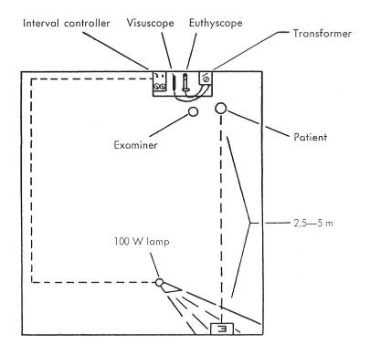
Proposal of accessories used with the Euthyscope: Intervall controller (Please indicate voltage) Transformer for Euthyscope and Visuscope, 6 V 2,5 A adjustable to 4—9 V Chart with E-letters on paper Pointer for children
