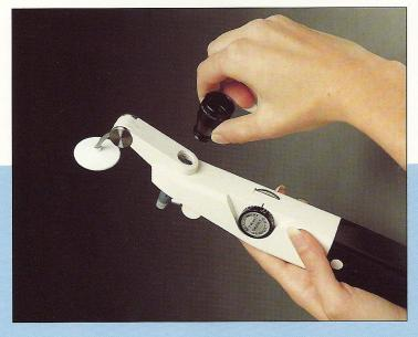
The Perkins Tonometer has been established for over 20 years as a "world standard" in hand-held applanation tonometers.
