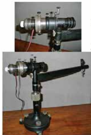
Fig. 2. Complete set of apparatus for eye hospitals: Slit Nitra lamp with Koepple diaphragm tube, polariser, revolving coloured glass wheel and non-spherical aplanatic Vogt slit lamp lens with adjustable Koepple silvered mirror, and Koepple eye microscope with single objective, analyser and binocular attachment for ultra-microscopic and micro-polariscope observations. Above this: A Vogt slit arc lamp (interchangeable with the Nitra lamp) with cooling cell, Koepple diaphragm tube with polariser, and double revolving wheel with smoked glasses and coloured glasses, with non-spherical aplanatic Vogt slit lamp lens and adjustable Koepple silvered mirror (about \frac{1}{2} act. size).
