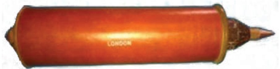
240volt hand held electromagnet for extracting ferrous foreign bodies
