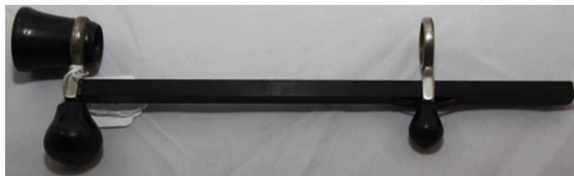
Above: Simple optometer (c1870) consisting of a single convex lens and a movable target
